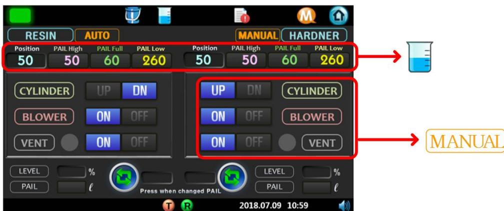
The pail page is a page for the manual operation the set-up of the pail. It is possible to operate the screen touch and the switch of the front panel of the equipment on the pail page.
