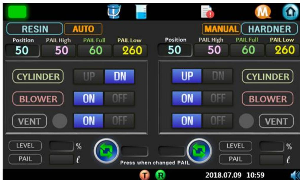
During manual replacement of pail, the replacement can proceed to manual mode by referring to the auto mode sequence on pail page.
