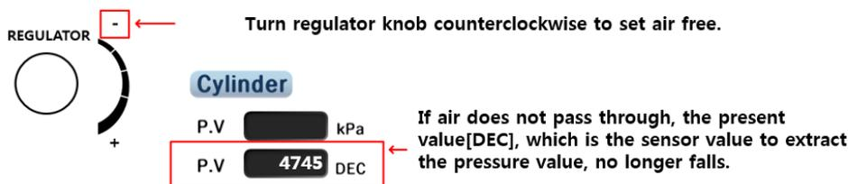
Recognize that the extraction sensor value is 0kPa and set the minimum value as below.
