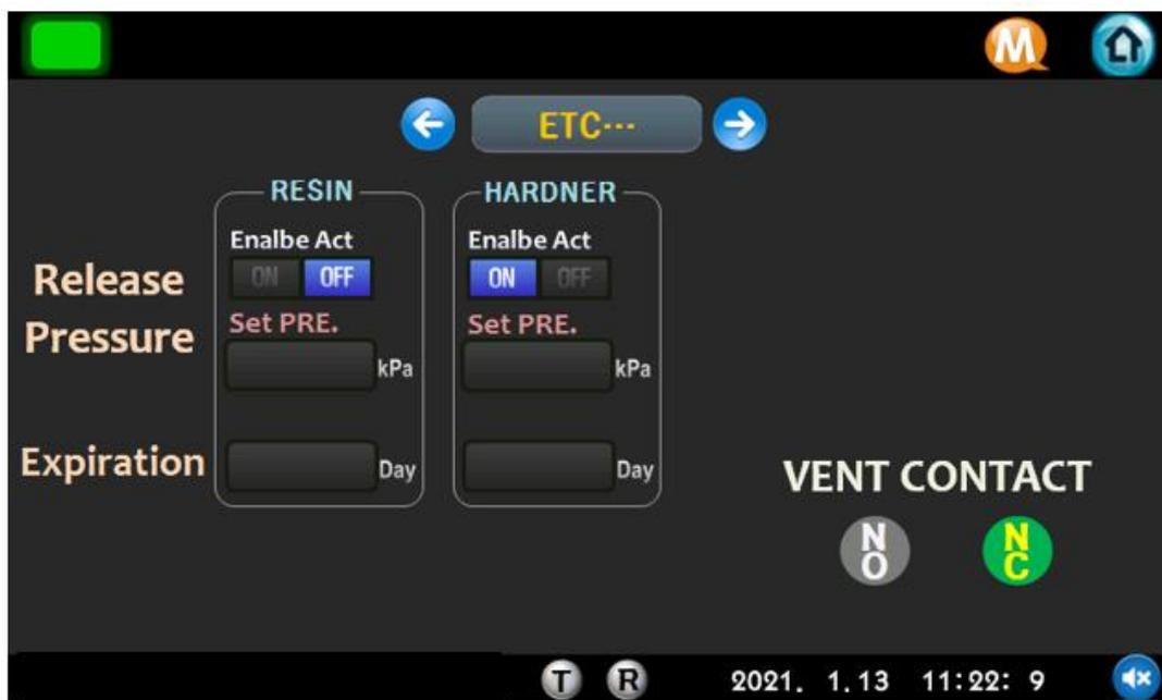
Release Pressure function (option), Expiration (liquid expiration date Japan-Korea) function, Vent contact setting (setting before factory shipment) screen.
