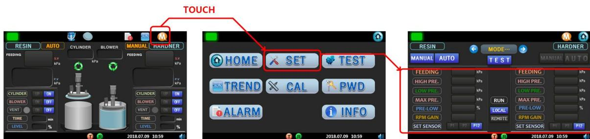
Once the material container has been combined, set the liquid transfer conditions as shown above and proceed to the Home screen to prepare for the start of liquid transfer.
