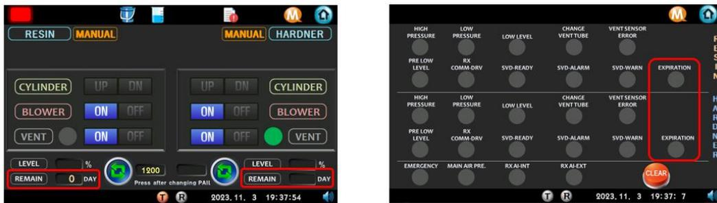
After the remaining time period, the manual home screen displays an alarm after the date.
