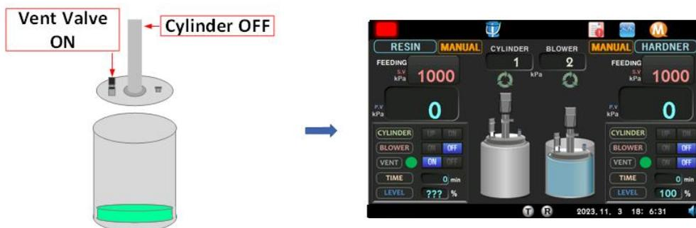
Vent valve is turned off automatically, and Level is displayed as "???"
