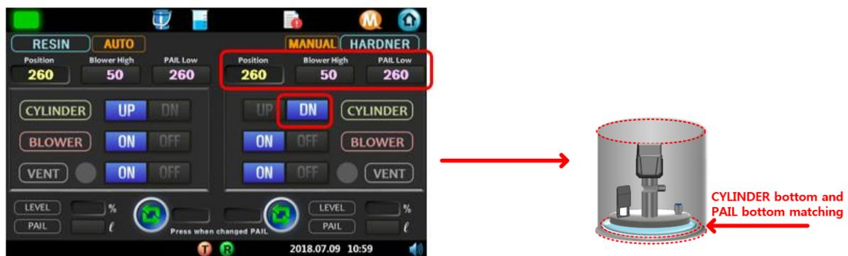
Lower cylinder operation pressure to minimum (150 ~ 200kPa) to minimize cylinder movement speed.
