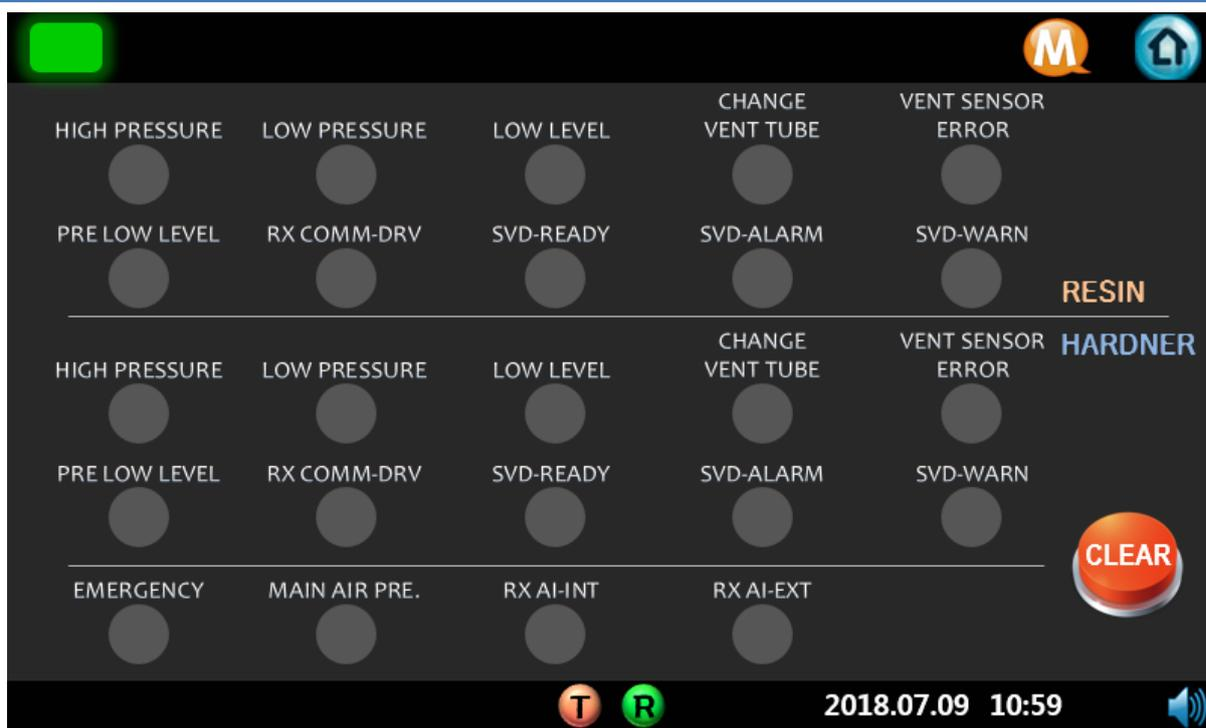
This page shows the alarm when there is a problem with using PRO-CPD20. The alarm description and action for each item are as follows.
