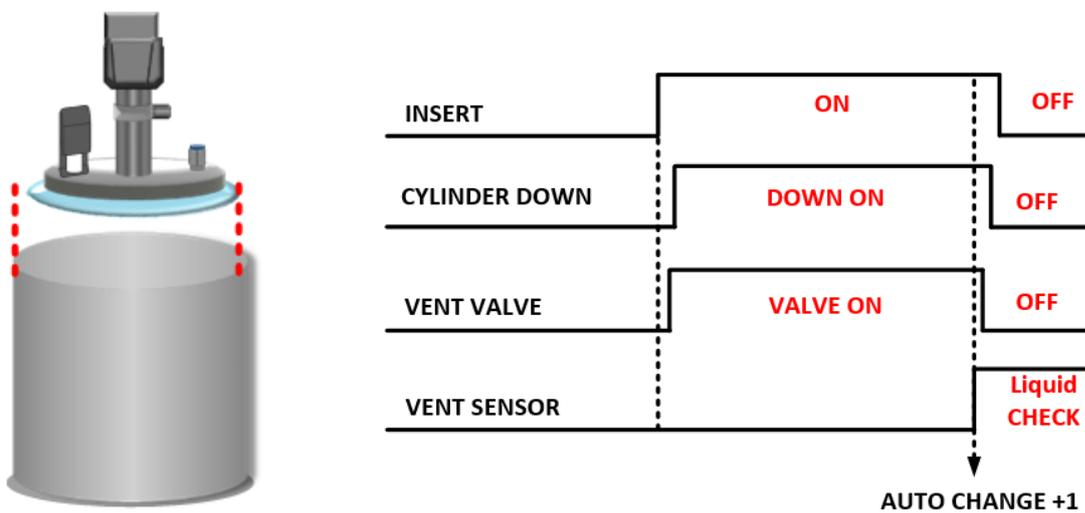
Refer to the figure above, align the Pail in the same way as the upper follow plate, and then click the insert button in the auto mode state.
