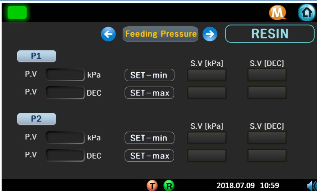
This screen is for calibrating to set the information required for the sensor. (It will be shipped after setting is completed.)
