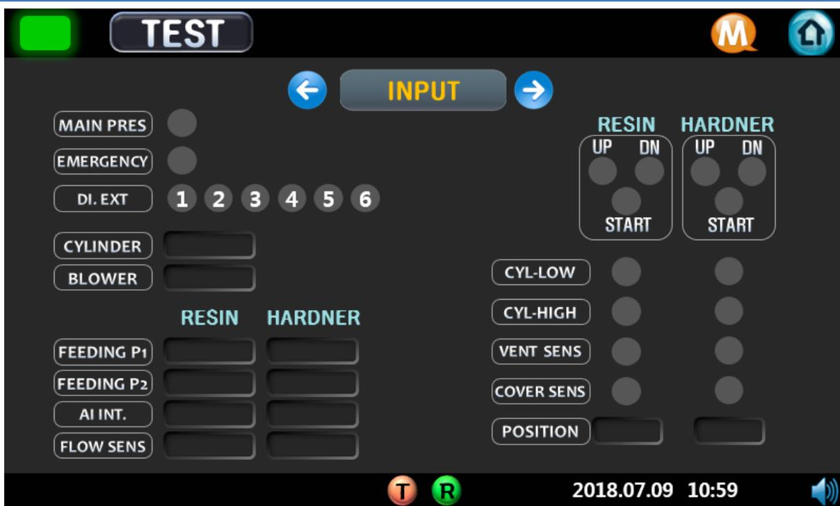
This page is to check PRO-CPD20 input contact point and sensor value.
