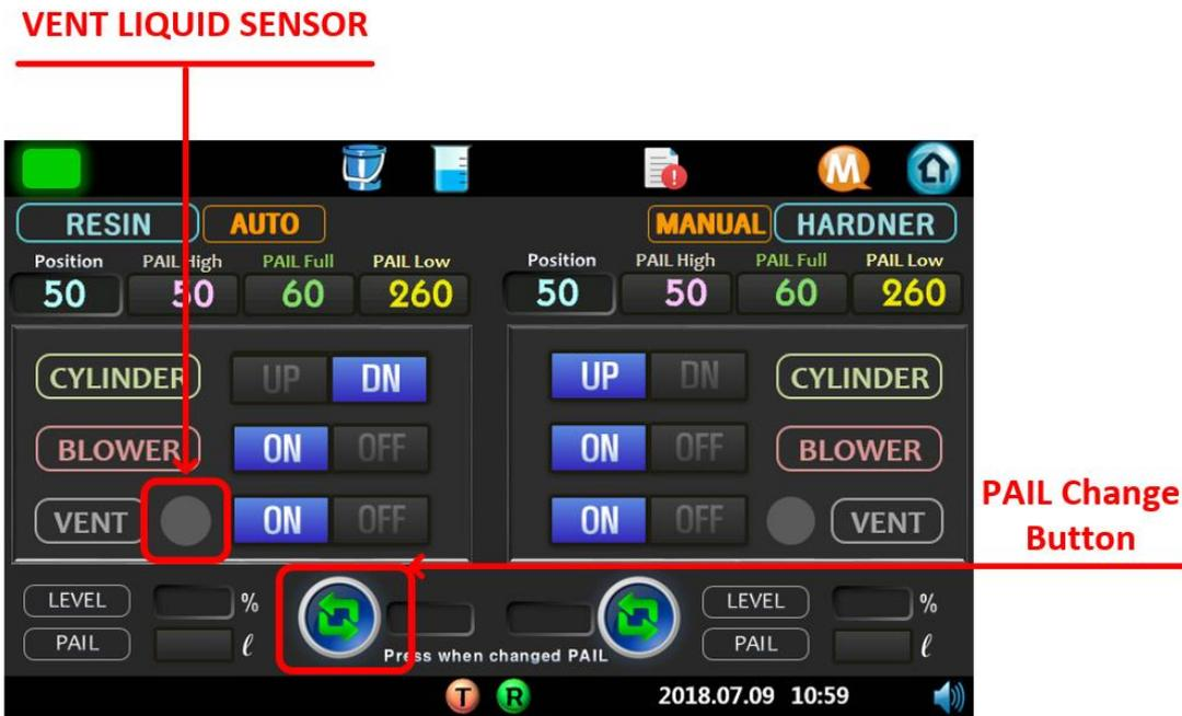
Change the current setting mode to manual mode, and then assemble the pail.
