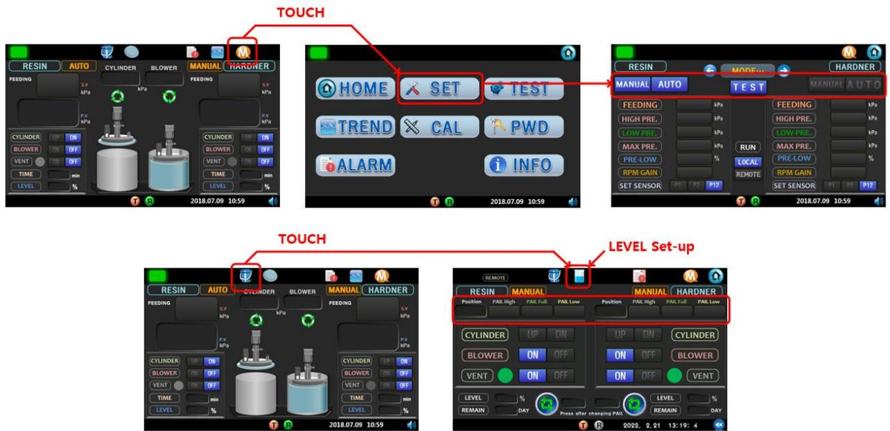
Go to the setting mode as below, switch to manual mode, and touch the cylinder level operation icon on the manual operation page to prepare the initial material container setting. (The initial password when entering the SET PAGE is 0000.)
