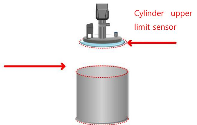
Raise the cylinder on the manual operation screen to reach the cylinder top sensor.
