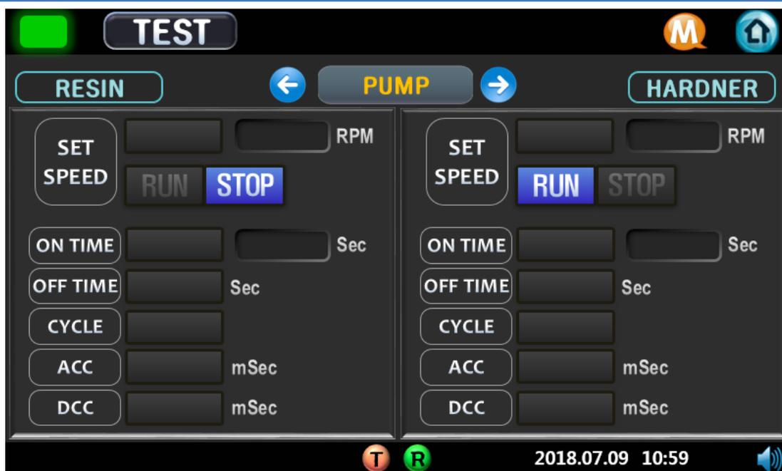
This page is the page for executing pump test. The equipment can be switched to test mode from this test page, and this page can be accessed with the administrator password.
