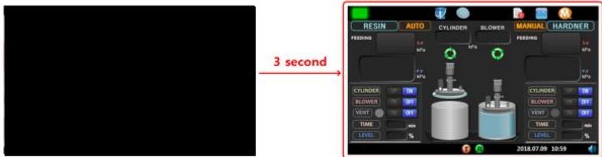
If power is applied after connecting the PRO-CPD20 power connector, the display will show the home screen after the intro screen display for 3 seconds as follows, and information will be activated on each display window.
