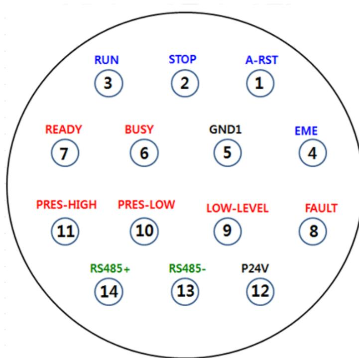
Pin map applied when using external I/O connector.
