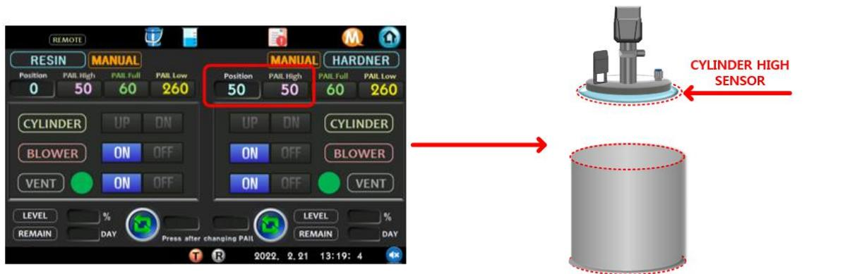
Raise the cylinder on the manual operation screen to reach the cylinder top sensor.
