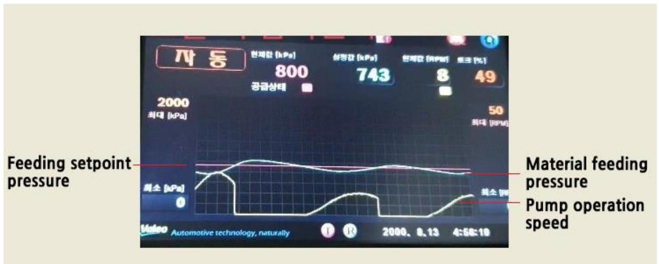
(Example: Real disply for feeding setpoint pressure, material feeding pressure and pump operation speed)
