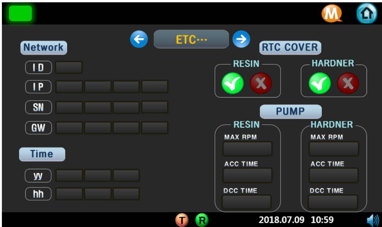
This is the set page(etc.) for setting upper-level communications, RTV cover selection (vacuum type), time setting and pump speed setting.
