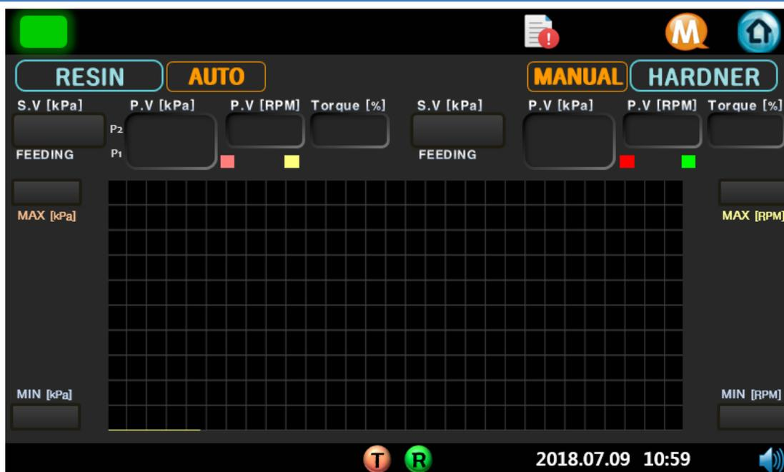
When operating the equipment, you can check the supply pressure and motor information via a real time graph.
