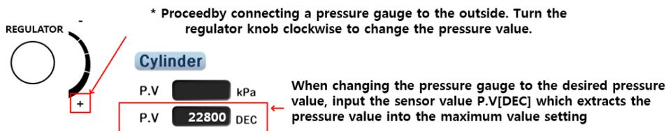
Set the set pressure gauge value and pressure sensor extraction value to the maximum value as shown below.
